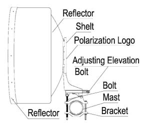
Installation Instruction: 1. Assemble the feeder to the installation bracket, and adjust the polarization mark of feeder and installation bracket. 2. Install the antenna on the holding pole with the mounting kids, adjust the direction, tighten the nut, makes the antenna fixed around the holding pole (Note: the side with osculum around the reflector should be downward) .3. Adjust direction, elevation and nut, make the antenna aim at the direction that with maximal signal and require to cover.
